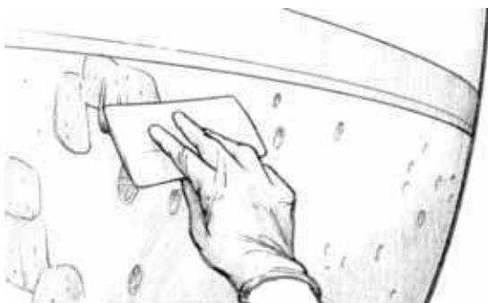
Figure 6.2 Use a squeegee to apply fairing compound, and slightly overfill the area. Shape the mix to blend with the surrounding contour.
